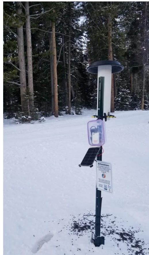
Figure 1. Rosy-finch study feeder design. Note black loop antennas on the perches, electronics box, and solar panel.
